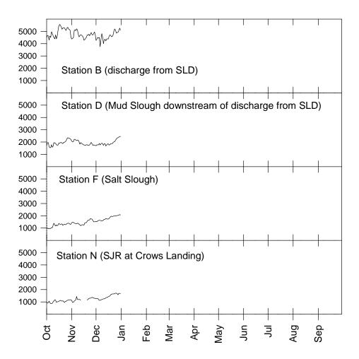
Figure 10. Specific conductance ( $\mu$ S/cm) in weekly grab samples. Letters indicate stations.
