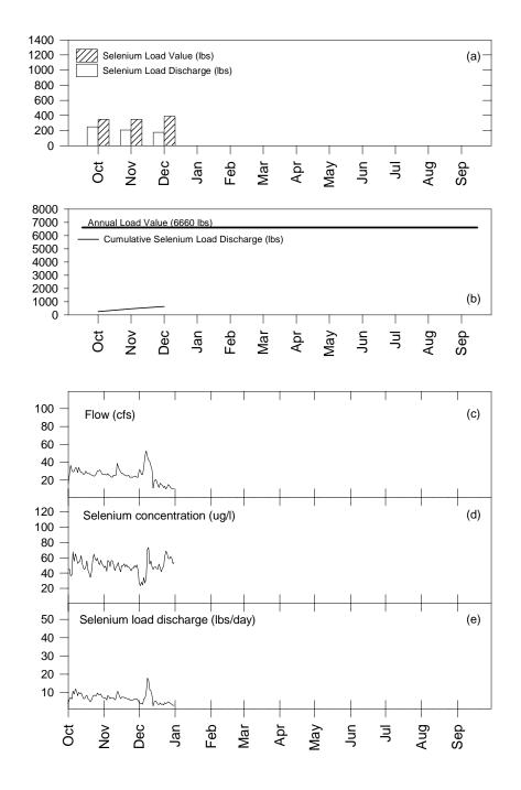
Figure 5. Daily average flows and selenium concentrations at station N (San Joaquin River at Crow's Landing). Flows at station N for January and February were estimated (see text). Note break in vertical axis for flow plot.
