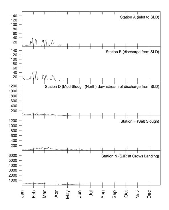
**Figure 2.** Comparison of monthly selenium load discharge from the terminus of the San Luis Drain (Station B) with the monthly load values in the Interim Use Permit for calendar year 2015.
