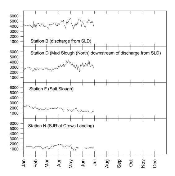
**Figure 9.** Specific conductance ( $\mu$ S/cm) in weekly grab samples. Letters indicate stations. Station H data intended for use with biological monitoring data.
