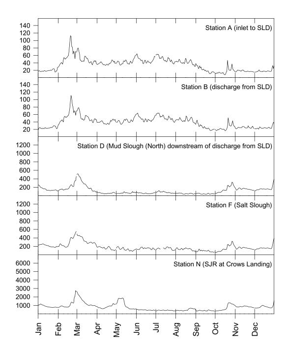
**Figure 2.** Comparison of monthly selenium load discharge from the terminus of the San Luis Drain (Station B) with the monthly load values in the Interim Use Permit for calendar year 2004.
