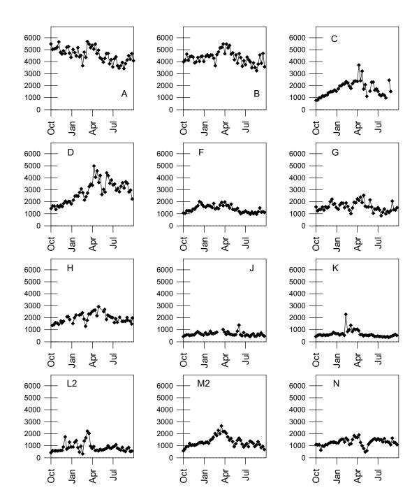
Figure 9. Specific conductance ( $\mu$ S/cm) in weekly grab samples. Letters indicate stations. Station H data intended for use with biological monitoring data.
