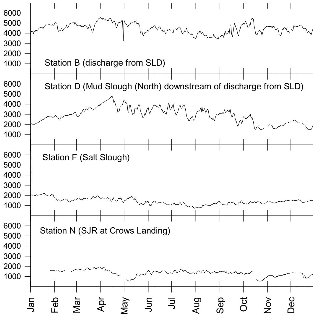
**Figure 9.** Specific conductance ( $\mu\text{S}/\text{cm}$ ) in weekly grab samples. Letters indicate stations. Station H data intended for use with biological monitoring data.
