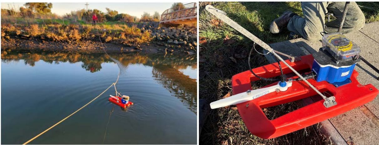
Figure 5. StreamPro ADCP Used to Collect Transects in Shallow Water.
