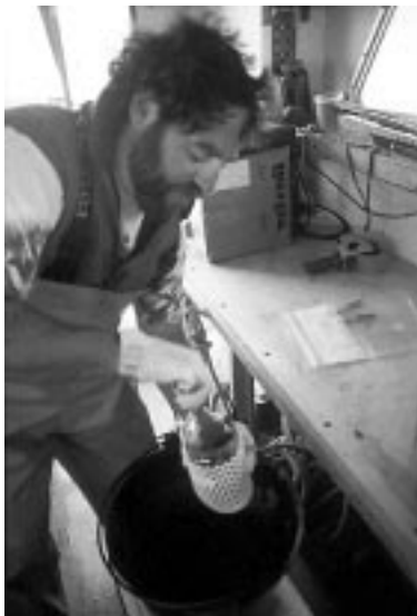
Sub-sampling sediment from a composite sample. Sediment sampling is conducted using a modified Van Veen grab. The top 5 cm of sediment is scooped from each of two replicate grabs and mixed in a bucket to provide a single composite sample for each station. The sample is divided on board for each analytic laboratory and for sediment toxicity tests.
