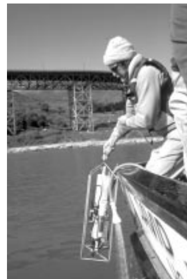
Using the Sea-bird SBE19 Conductivity, Temperature and Depth probe (CTD). The CTD measures water quality parameters at depths throughout the water column. Casts are taken at each site during water and sediment sampling.
