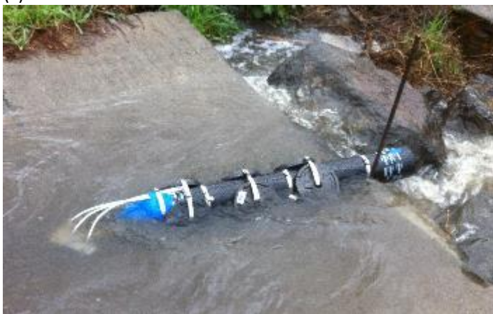
Figure 2. Sampling equipment used in the field. (a) Painter's pole, Teflon tubing and an ISCO used as a slave pump; (b) Teflon bottle attached to the end of a DH81 sampling pole; (c) a Walling Tube suspended sediment sampler secured by 5-lb weights along the body of the tube (because it is sitting atop a concrete bed) and rebar driven into the natural bed at the back of the sampler; and (d) a Hamlin Sampler.
