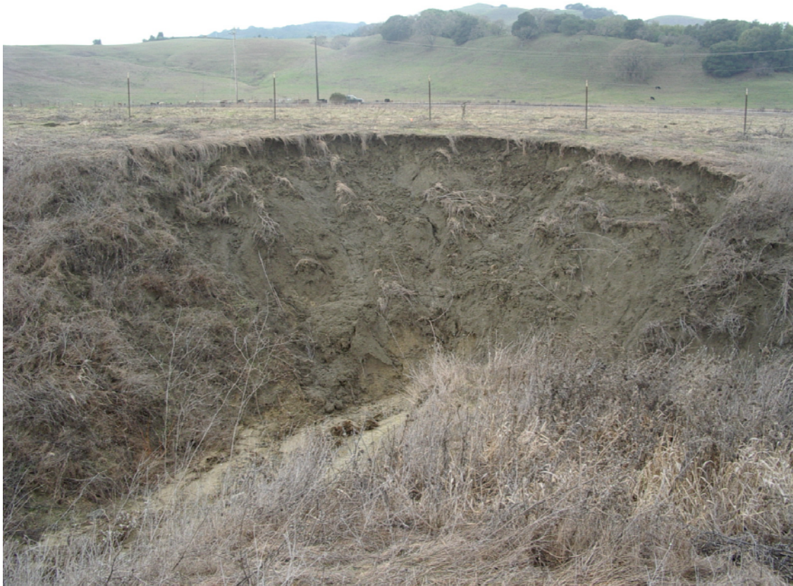
Figure 22. Photograph showing the bank erosion occurring on the left bank of BXS2.
