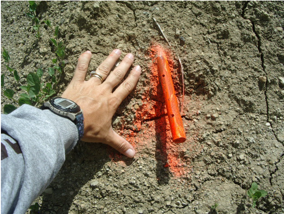
Figure 25. Photograph of exposed bank pin at AXS3, May 2006.
