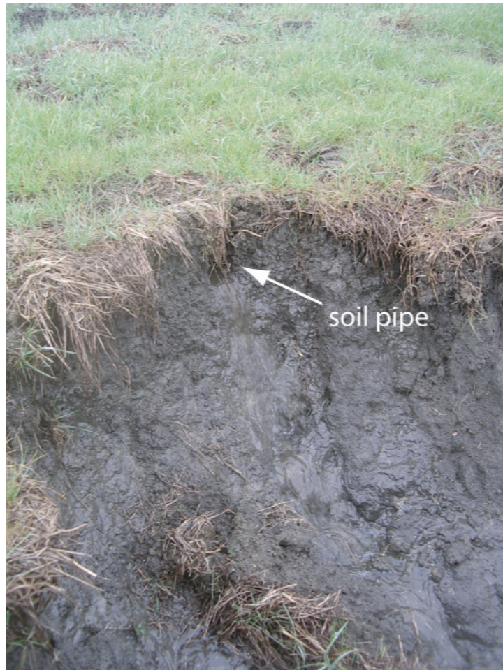
Figure A-4. Photograph of soil pipe discharging water into a gully channel.
