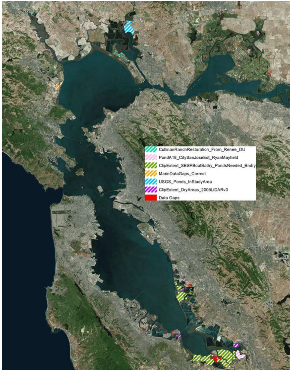
Figure A1. Locations of topobathymetric data appended to flat areas of the DEM used to determine polder fill volumes.
