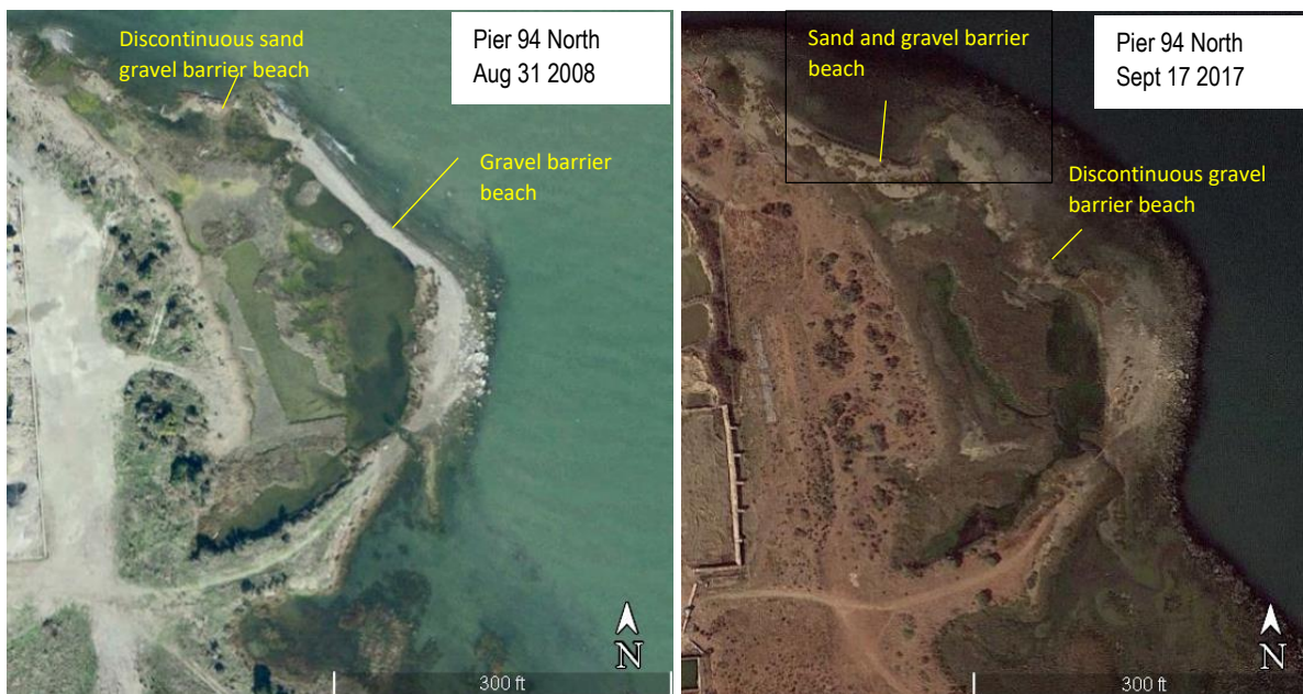
Figure 5. Pier 94 north shore sand and gravel barrier beach evolution. The outer northeast-facing linear gravel barrier beach (2008) migrated landward into the lagoon and became a diffuse, discontinuous gravel beach veneer by 2017. Sand and gravel drifted west as the outer barrier declined, and consolidated an enlarged western barrier beach that welded with the backshore by 2017.
