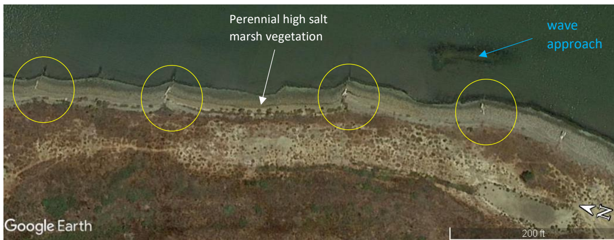
Figure 12. Short backshore groins (“micro-groins” or drift-sills; yellow circles), constructed from decay-resistant logs and boulders, provide persistent local obstructions to longshore drift of beach gravels, causing subtle beach protuberances and updrift beach accumulation wedges at intervals along the shoreline. Relatively stable storm gravel beach ridge positions between micro-groins are ecologically indicated by patchy growth of perennial high salt marsh vegetation along their crests.
