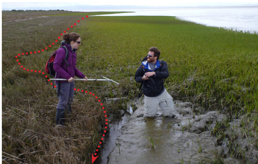
Figure 4. The mapped shoreline. The red-dotted line in this field photo corresponds to the boundary between the consolidated marsh plain and unconsolidated cordgrass-dominated low marsh (where staff sunk up to their knees). Photo taken along the Highway 37 marsh in Solano County (photo by Julie Beagle, April 2012).
