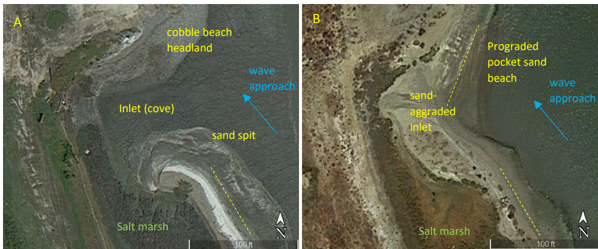
Figure 11. Aramburu Island, central shore cove, evolution from drift-aligned spit towards swash-aligned pocket beach. (a) Newly nourished sand spit at south end of cove in 2012, oriented southeast-northwest (dashed yellow line). Cobble beach headland faces southwest at the north end of the cove. (b) Sand spit progradation in 2018 (following strong net sand drift 2012-2018) fills in the cove, and a new sand beach reoriented southwest-northeast (dashed yellow line) forms in the pocket along the former cobble beach headland, facing prevailing wave approach from the southeast, refracted within the cove. Images: Google Earth.
