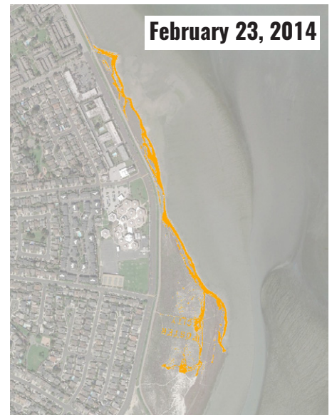
Figure 5. Foster City beach is a complex of spits and a marsh-fringing barrier beach with a southward migration over time, as captured for eight time steps from 2003 to 2018. Foster City beach separates into two parts between 2003 and 2007, and connects between 2008 and 2018.
