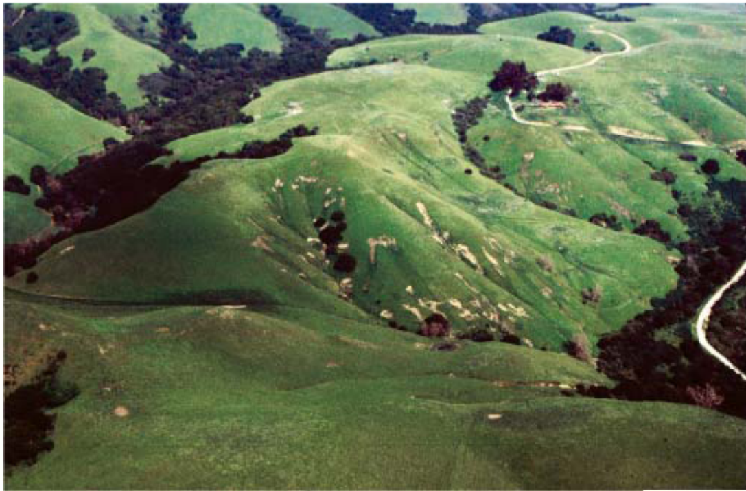
Appendix Figure 11. Photograph illustrating 1998 debris flows on Walpert Ridge (from Coe and Godt, 2002).
