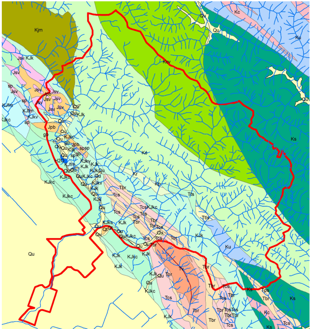
Appendix Figure 2. Bedrock geology underlying the Dry Creek watershed (Graymer et al, 1996). Major units include: Ko (Oakland sandstone), Kcv (Unnamed sandstone, conglomerate, and shale of the Castro Valley area), Ks (Unnamed sandstone and shale), Kjk (Knoxville Formation silt or clay shale with thin sandstone beds), Qu (surficial deposits, undivided), Tbr (Briones Formation, sandstone, siltstone, conglomerate), Tcs (Claremont Shale), Jsv (Keratophyre and quartz keratophyre), Kjm (Joaquin Miller Formation thinly bedded shale), Jpb (pillow basalt), Jb (massive basalt), Jgb (gabbro), and sp (serpentine).
