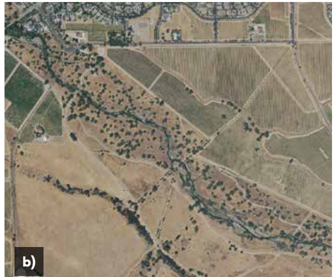
Figure 22. Aerial imagery comparison for the area that is now Sycamore Grove Park along Arroyo del Valle. In a), the 1939-1940 imagery shows a braided channel pattern with large areas of bare sediment (light signature), indicating regular disturbance by high flows. These signatures are largely absent in the post-dam imagery (2018, courtesy NAIP).
