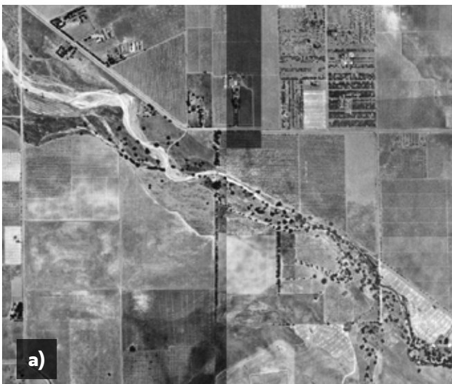
Figure 23. Aerial imagery comparison for the reach where the Wentz Vineyard sites are located along Arroyo Mocho. In a), the 1939-1940 imagery shows the wider active channel, evidence of meandering, and side channels in comparison to a narrower stream corridor in the contemporary imagery (2018, courtesy NAIP).
