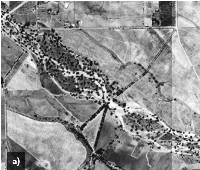
Figure 22. Aerial imagery comparison for the area that is now Sycamore Grove Park along Arroyo del Valle. In a), the 1939-1940 imagery shows a braided channel pattern with large areas of bare sediment (light signature), indicating regular disturbance by high flows. These signatures are largely absent in the post-dam imagery (2018, courtesy NAIP).
