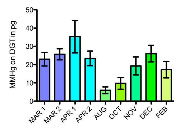
Figure 7: Seasonal variation of MMHg accumulation on DGTs at the Martin Luther King Regional Shoreline over the period from March 2009 to February 2010. Error bars represent standard deviation of replicate DGTs (n = 3). MAR 1+2 and APR 1+2 are two side-by side replicate deployments of two sets of DGTs, respectively, to evaluate the spatial variability of the DGT measurement at a single station.
