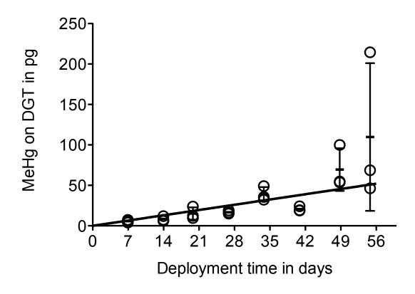
Figure 5: Accumulation of MMHg on DGT devices over an 8 week period. Linear regression shown is based on the entire 8 week period (ignoring the single high outliers observed at 7 and 8 weeks, respectively)
