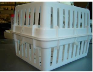
Figure 2: DGT piston configuration in bottom basket and closed DGT cage
