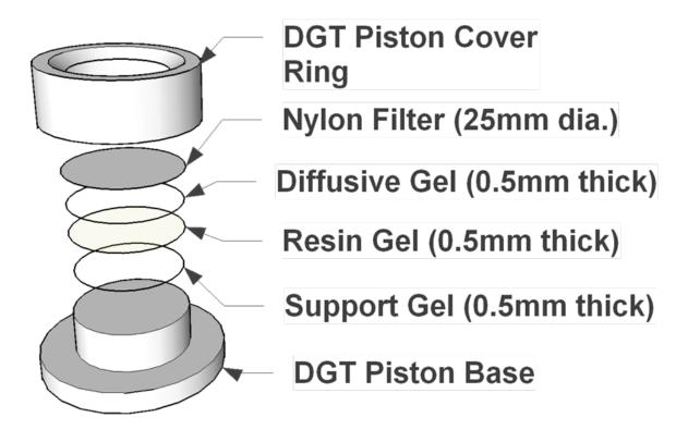
Figure 1: Water-DGT probe assembly
