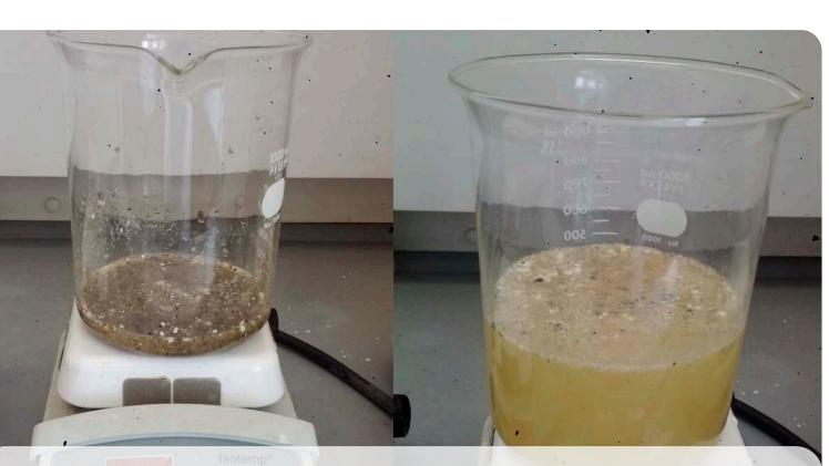
Wet peroxide oxidation (WPO) process: Before (left) and after (right) Photo courtesy Sherri A. Mason
