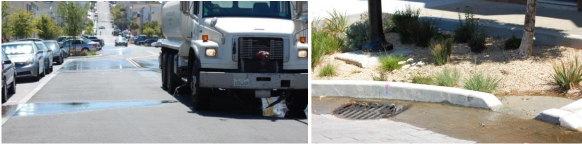
Figure 14. Images from water truck test in the summer of 2012 showing runoff bypassing the inlet to the bioretention planter and draining into the storm drain inlet.
