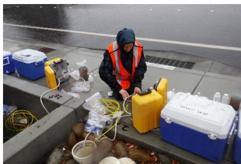
Figure 3. Inlet and outlet monitoring in the surface-loaded tree well (A) and outlet monitoring at the subsurface-loaded tree well (B) during a storm event.
