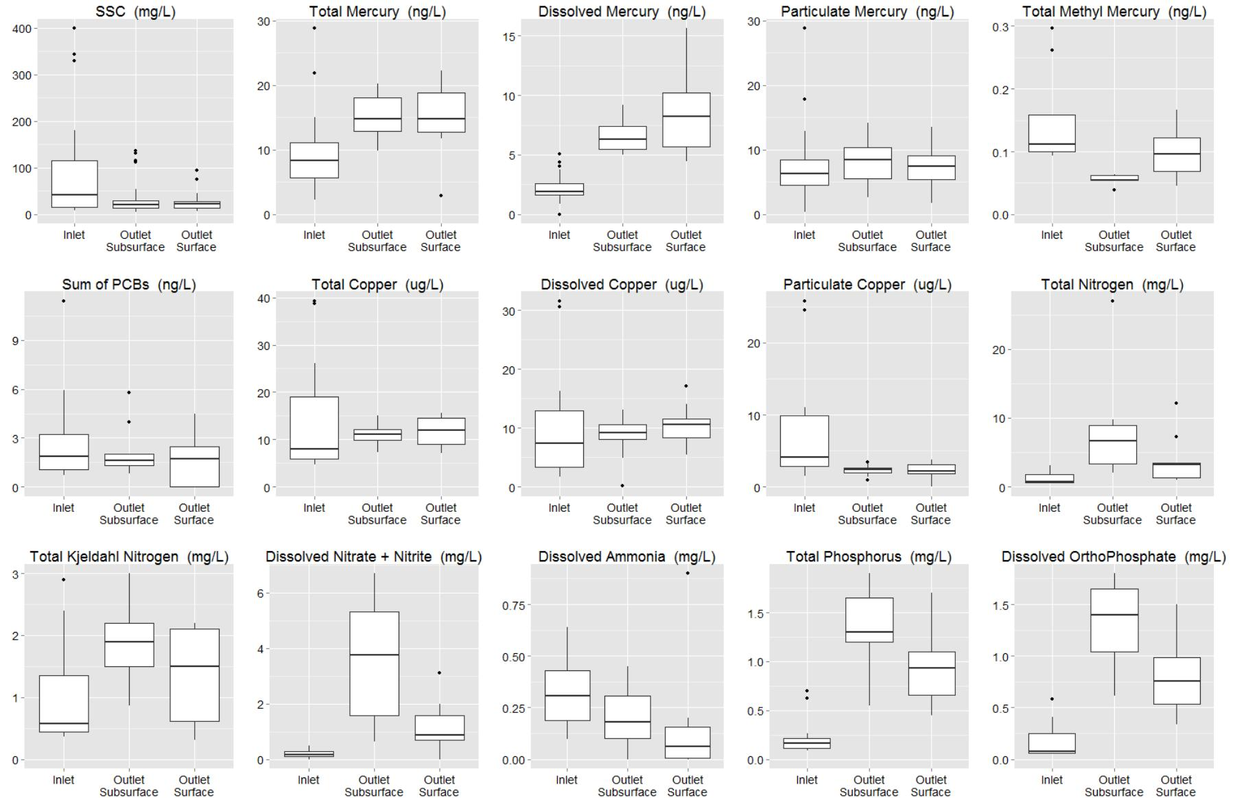
**Figure 5. Distributions of concentrations measured throughout the study at the inlet (data from both tree well filters combined) and each TWF outlet. Note: see call-out box on previous page for details on how to read a box-and-whisker plot.**
