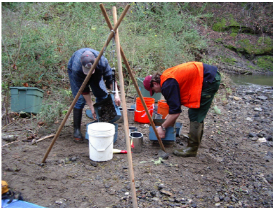
Figure 6-17. Two of the eight Gilson metal sieves used in the field for bulk sediment sampling.
