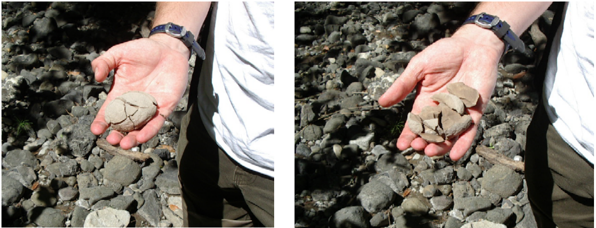
Figure 6-15. Photographs of a clast of mudstone from the bed, commonly found in parts of Segment III. Upon wetting and drying, these rocks readily decrepitate into smaller fragments.
