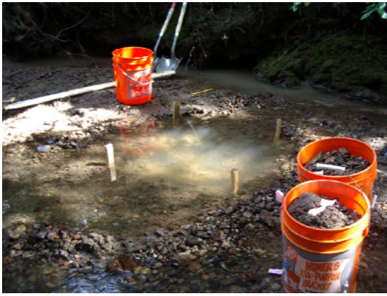
Figure 6-16. An excavated bulk sediment sample site. Wood stakes define the boundary of excavation.
