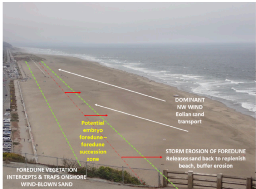
Figure 8.3. Diagram of natural sand transport processes along Ocean Beach. Regular beach grading north of Lincoln interrupts these processes and limits the natural development of embryo foredunes.
