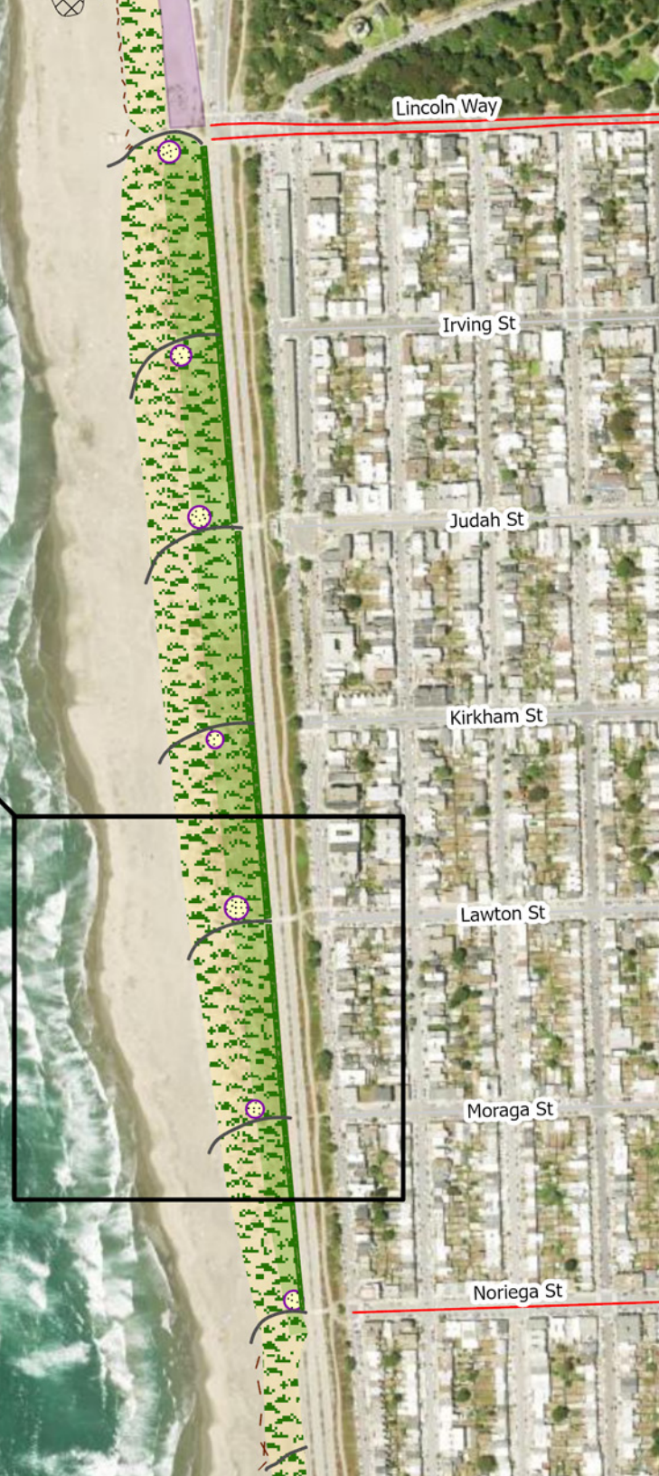
Figure 8.5. Concept design summary for Reach B. Reach B design elements focus on revitalizing the existing dunes and guiding pedestrian access to designated locations to reduce trampling.
