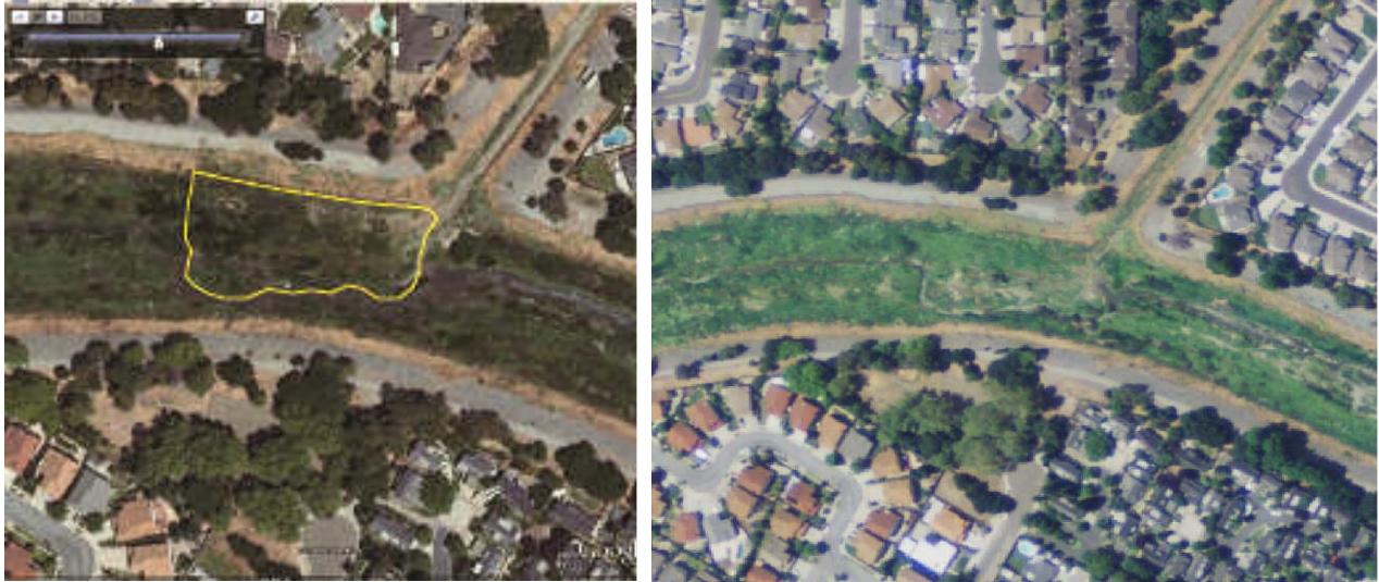
Figure 6. Left: Aerial photograph showing the fan (outlined in yellow) formed within the Alameda Creek flood control channel by Dry Creek, as shown in 2007. Flow in Alameda Creek is from right to left. Right: 2009 aerial photograph showing the same location; Alameda Creek low flow channel is clearly deflected towards the left bank due to the Dry Creek fan.
