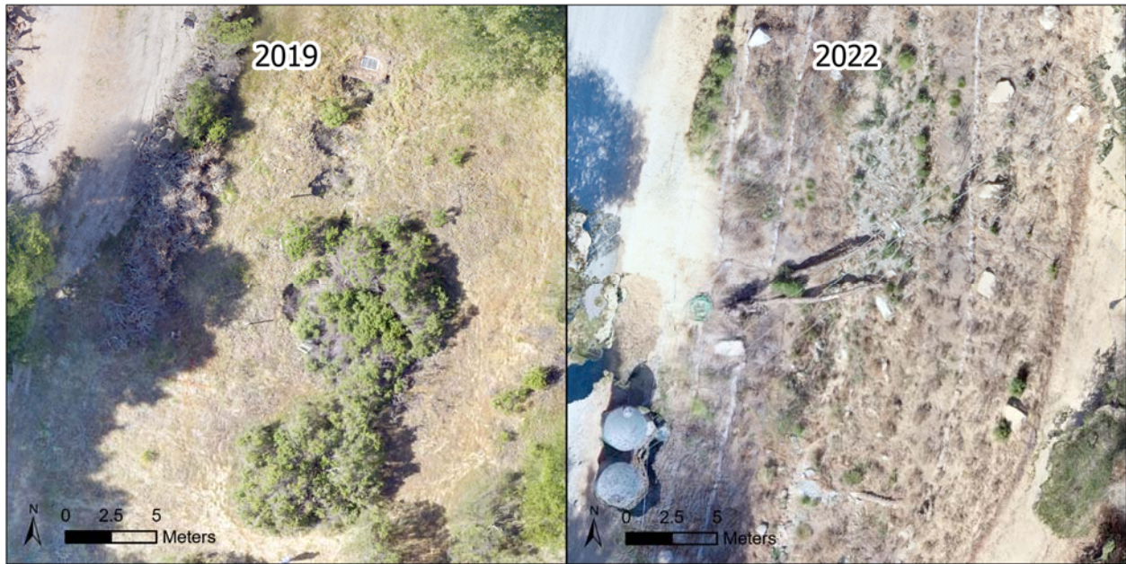
Figure 32. Comparison of the valley morphology in 2019 with visible sinkholes due to the failing culvert, with the 2022 valley morphology that features the newly created channel.
