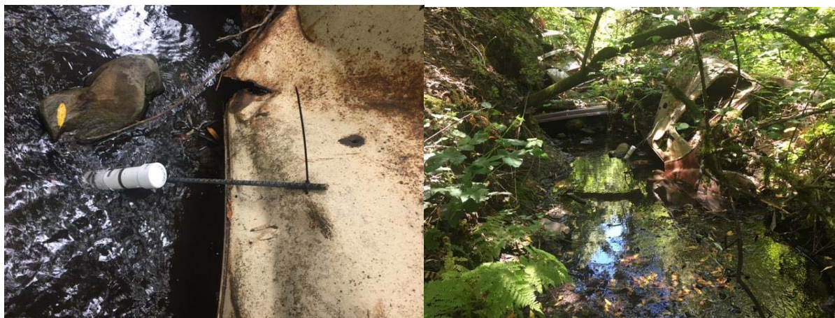
Figure 7. 2020 temperature sensor deployment in Upper San Leandro Creek. Left: PVC housing attached to rebar sticking out of the water near an old car body. Right: Looking upstream at the old car body. The PVC is just visible in the middle of the picture. June 11, 2020.
