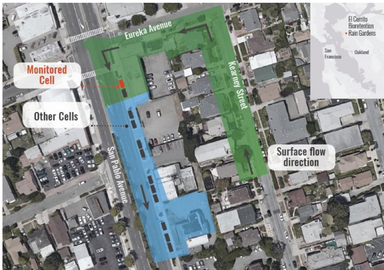
Figure 1. Map of the watershed area draining to the El Cerrito Rain Gardens. The upper watershed (green, 4080 m 2 ) drains to the monitored cell. The lower watershed (blue) drains to the other rain garden cells, which also receive overflow and bypass from the monitored cell. The monitored cell and adjacent cell drain to a common subdrain.
