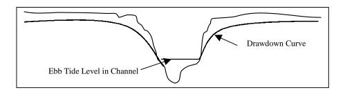
The horizontal extent of the drawdown curve and the steepness of the curve indicate the extent and rate of tidal flushing of the bank sediments.
