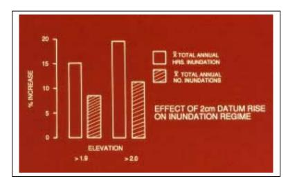
The chart at left says that a 2 cm rise in high tide (or a 2 cm drop in marsh elevation) causes a 15% increase in hrs of inundation at 1.9 m above low tide, and a 20% increase at 2.0 m above low tide. The source of data is a study I did of the effects of mosquito control ditches of tidal hydroperiod in Petaluma Marsh.
