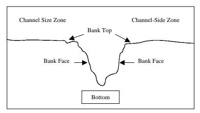
An important feature of the channel cross-section not shown in this diagram is the usual change in sediment type with distance away from the bank face. The channel bottom and banks mostly consist of inorganic sands, silts, and clays that are carried into the marsh and deposited by the tides. The amount of organic
