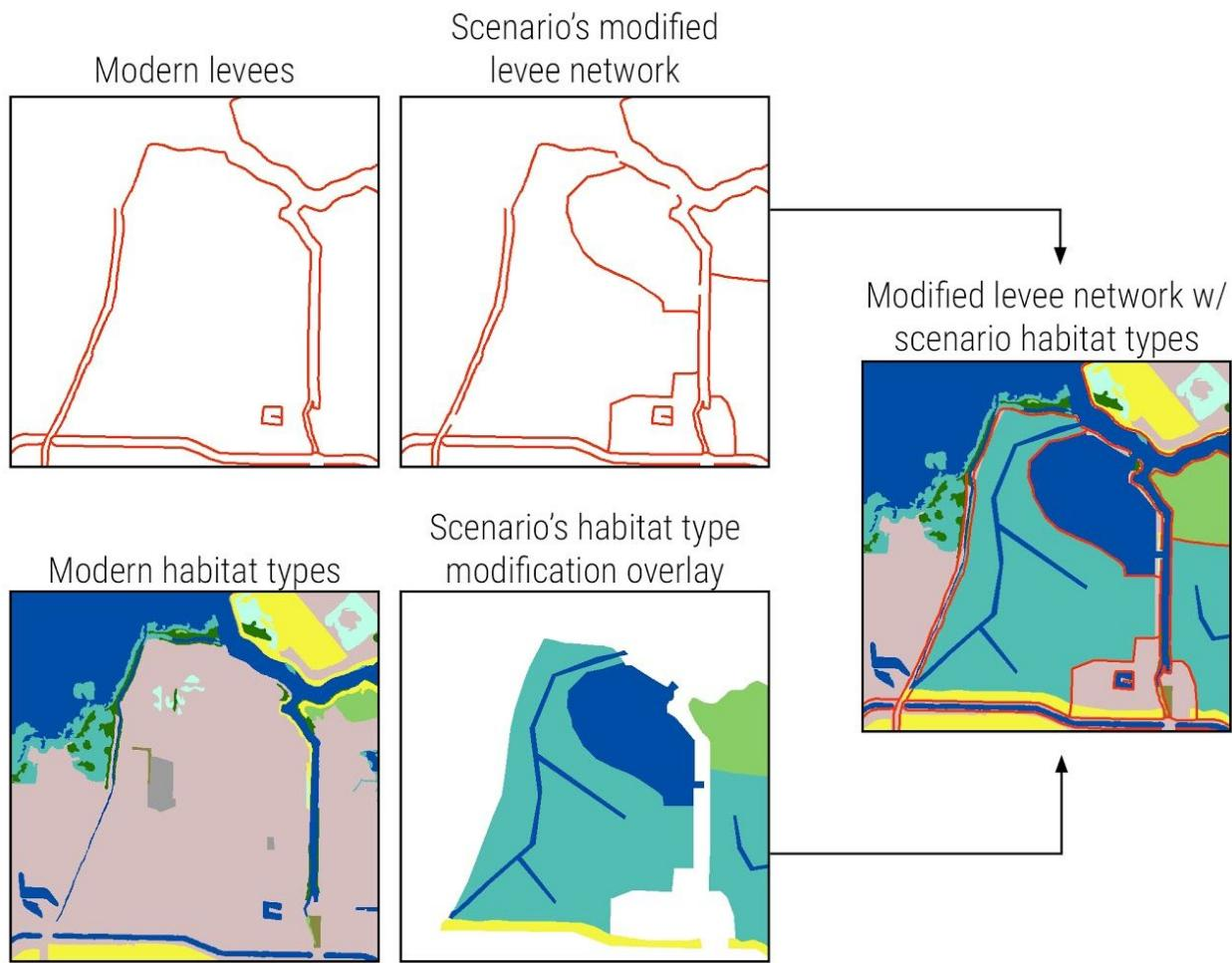
The levee network assigned to a scenario only impacts a subset of the modules and analyses run in the DLSPT. If the following analyses are not of interest to a particular user, the user does not need to provide a modified levee layer.
