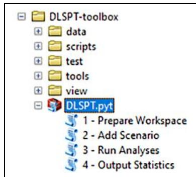
DLSPT consists of four specific tools. These are meant to be run in order, but certain tools can be repeated. Generally the procedure is as follows: (1) prepare the workspace, (2) add scenario(s) to the workspace, (3) run analyses, and (4) output statistics. The tool components and work flow are summarized in the figure below and described in detail on the following pages.
