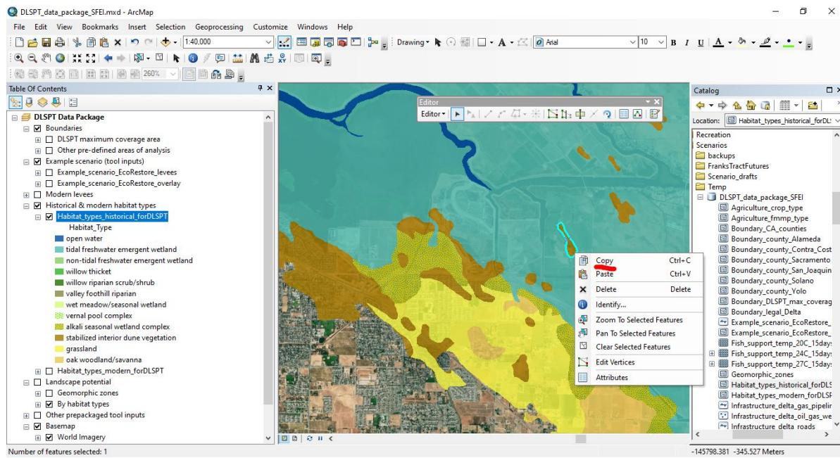
Step #2) Instructing ArcMap to paste this historical polygon into the example scenario habitat type modification overlay layer (CTRL+V with the scenario overlay layer turned on):
