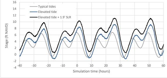
Figure 3. Discharge and tide boundary conditions for present and future hydrologic scenarios
