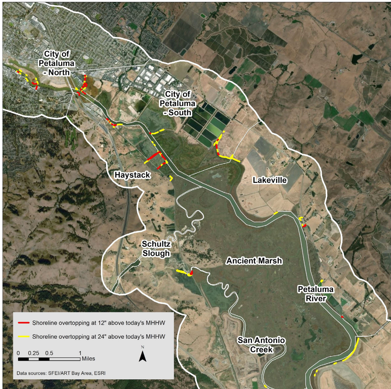
Figure C-12. Shoreline overtopping at 12" and 24" above today's MHHW for selected levees in the northern half of the study area. Segments symbolized in the map were selected based on proximity to main channels and diked baylands. Some segments shown are not the first line of defense and therefore may not be subject to overtopping at these levels unless external levees are compromised.
