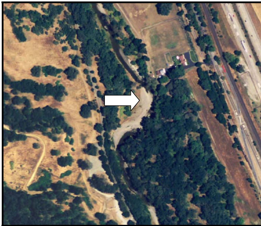
Figure 73. 2005 aerial photograph showing a point bar adjacent to an actively failing erosional bend at bank stabilization project site. Flow is from top to bottom.
