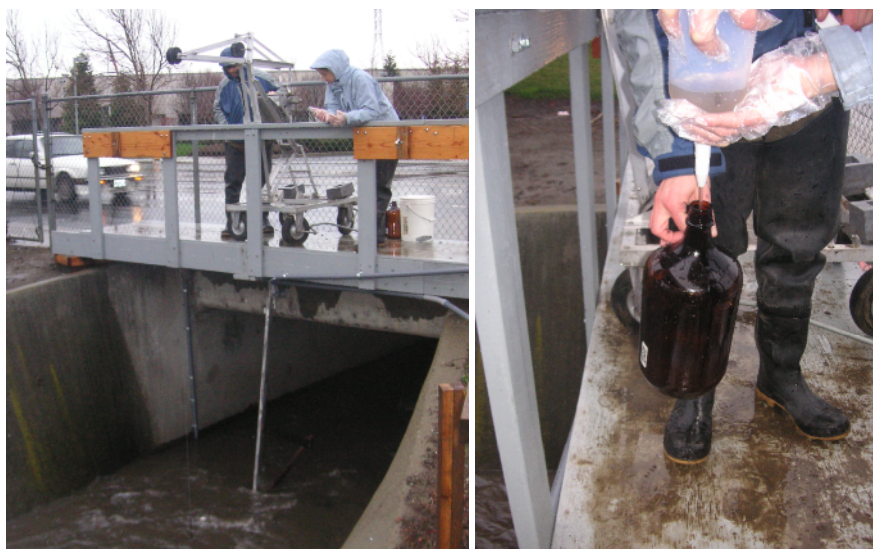
Figure 13. Lowering the D-95 sampler loaded with a 1-L Teflon sampling bottle into the channel during flood flow (picture at left), and decanting the bottle into an organics shipping bottle (picture at right).
