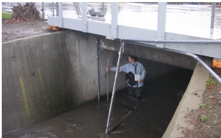
Figure 14. Measuring velocity at wading stage.
