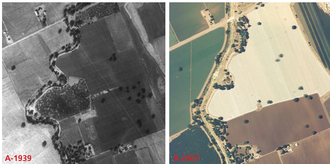
Figure 4.3. Former channel meanders of Llagas Creek. Over 60 km (40 mi) of historical streams (A) have been straightened or rerouted (B). Excavation of Llagas Creek in the early 1970s for gravel to construct Highway 101 and flood benefits produced these isolated oxbows along the current flood control channel (B; USDA 1982). (A: USDA 1939, courtesy of the Science & Engineering Library Map Room, UC Santa Cruz; B: USDA 2005, courtesy of NAIP)
