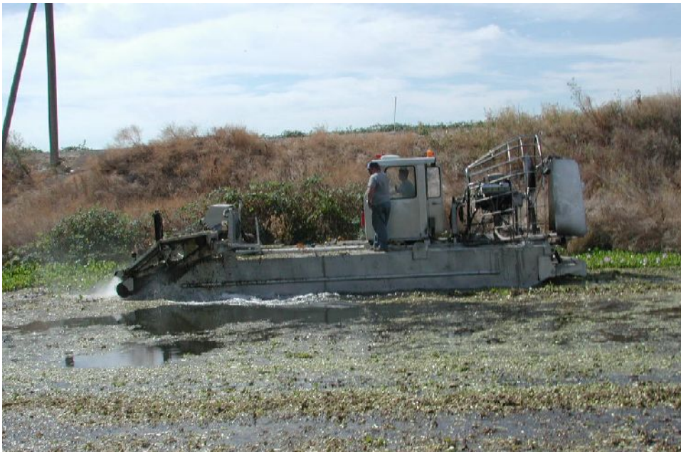
Figure 2. The Amphibian Terminator. Note the cut plant material in the foreground, uncut plant material in the background, and airboat fan on the rear of the vehicle.
