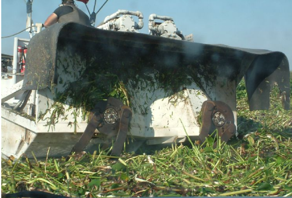
Figure 1. The AquaPlant Terminator, with a view of the rear cutting blades, engine, and cut plant material. Note that there is another set of cutting blades on the front end of the vehicle, which is similar in design to the Cookie Cutter (not shown). Photo credit: Bob Case, Contra Costa County Department of Agriculture.
