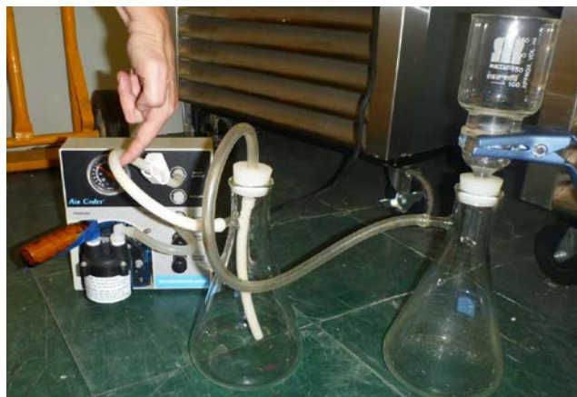
Figure 1. Filter setup for DOC/POC
