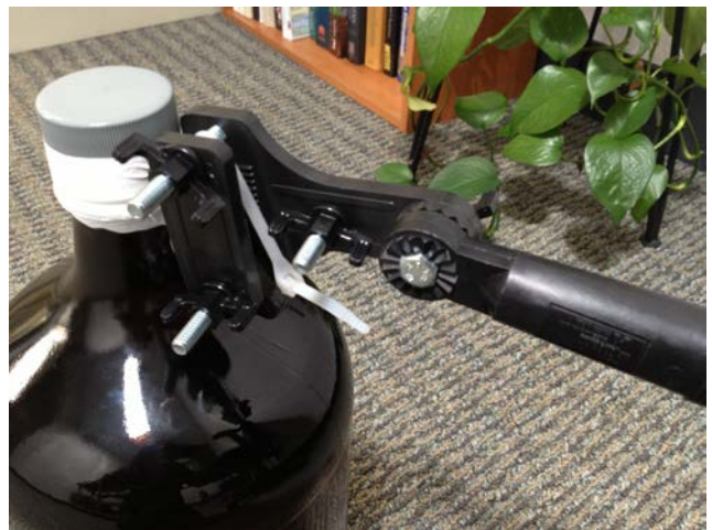
Figure 1: 4L recycled glass container attached to "tool holder" and telescoping grab sampler. String not included.
