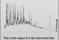
analyzed an Estuary water sample. Each spike, small or large, indicates the presence of a different chemical compound. One was identified as the pesticide diazinon. The vast majority remained unidentified.
