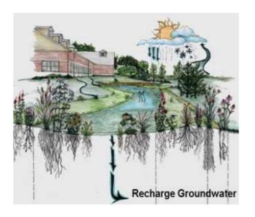
Runoff reduction is defined as the total volume reduced through canopy interception, soil infiltration, evaporation, rainfall harvesting, engineered infiltration, extended filtration or evapotranspiration
