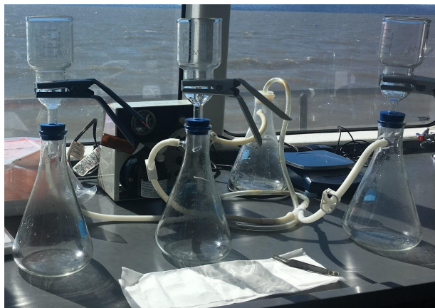
Figure 5. Particulate water sample filtration setup
