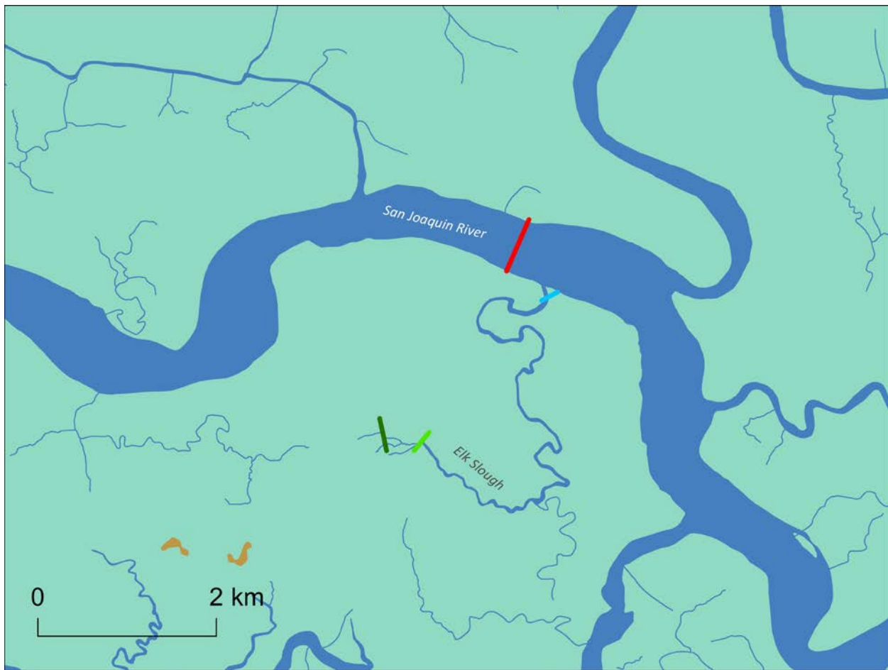
Figure 4. Modeled pre-development cross-sectionally averaged velocities from multiple points along Elk Slough (former Webb Tract blind tidal channel off of the San Joaquin River). Maximum velocities are substantially lower in the blind channel than in the mainstem river. See map for location of transects.
